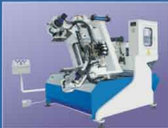
CASTING BY GRAVITY DIE CASTING MACHINE
